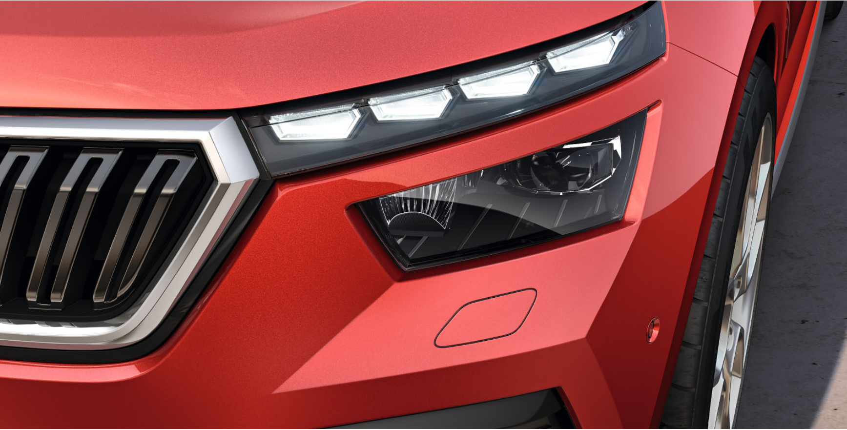
Bi-LED HEADLIGHTS The top-end option is all about LED technology including corner function and fog lights. The daytime running lights in the upper part of the two-piece headlights combines innovative technology with an unmistakable look.
