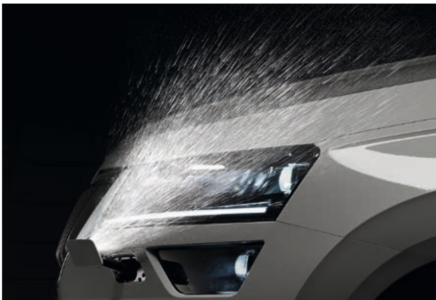
HEADLAMP WASHERS Integrated telescopic headlamp washers easily take care of dust and mud.
