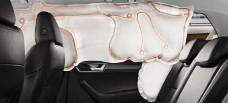
FRONT AND REAR SIDE AIRBAGS These four airbags protect the pelvis and chest of the driver and other passengers in the event of a side collision.
