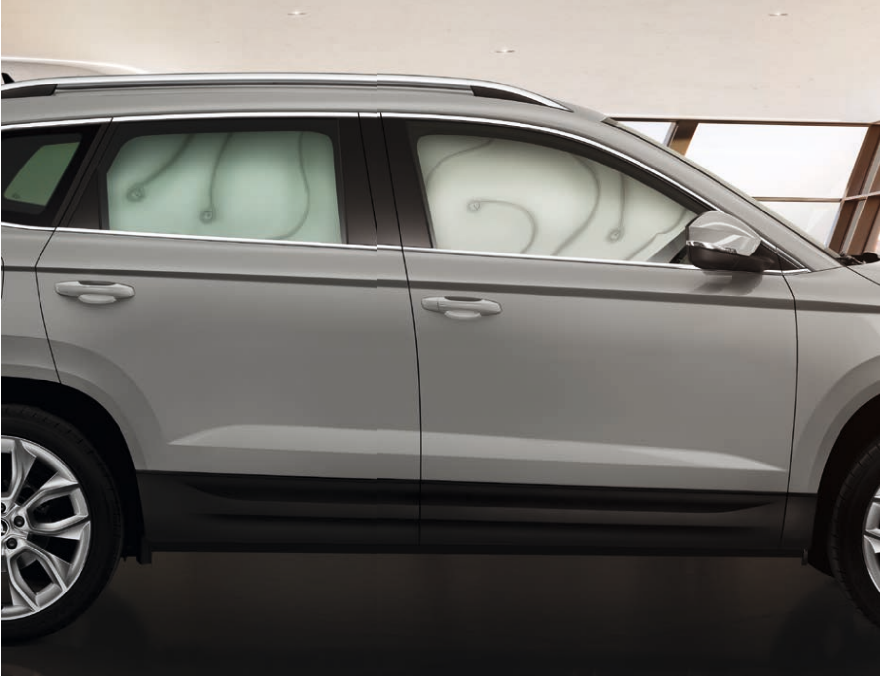
HEAD AIRBAGS Upon activation, head airbags create a wall protecting the front and rear occupants against head injury.
