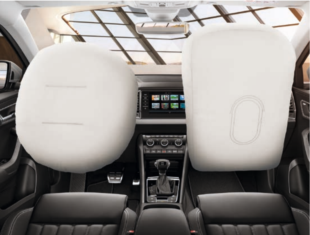
FRONT AIRBAGS While the driver airbag is enclosed in the steering wheel, the passenger airbag is located in the dashboard. If needed, this can be deactivated when a child seat is installed on the front seat.
