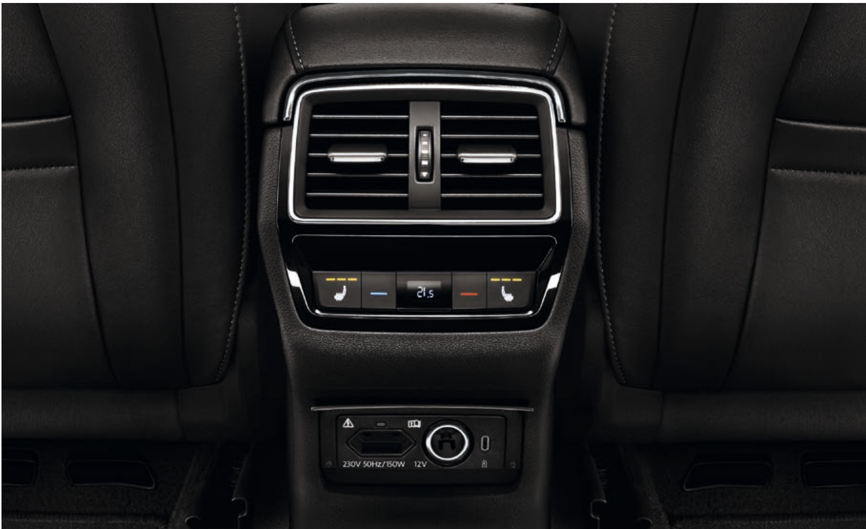
REAR PART OF THE JUMBO BOX On the rear part of the Jumbo Box you can find a 230 V socket and USC-C slot. In the car equipped with 3-zone Climatronic air conditioning, you will also find the control for the rear seat zone here.
