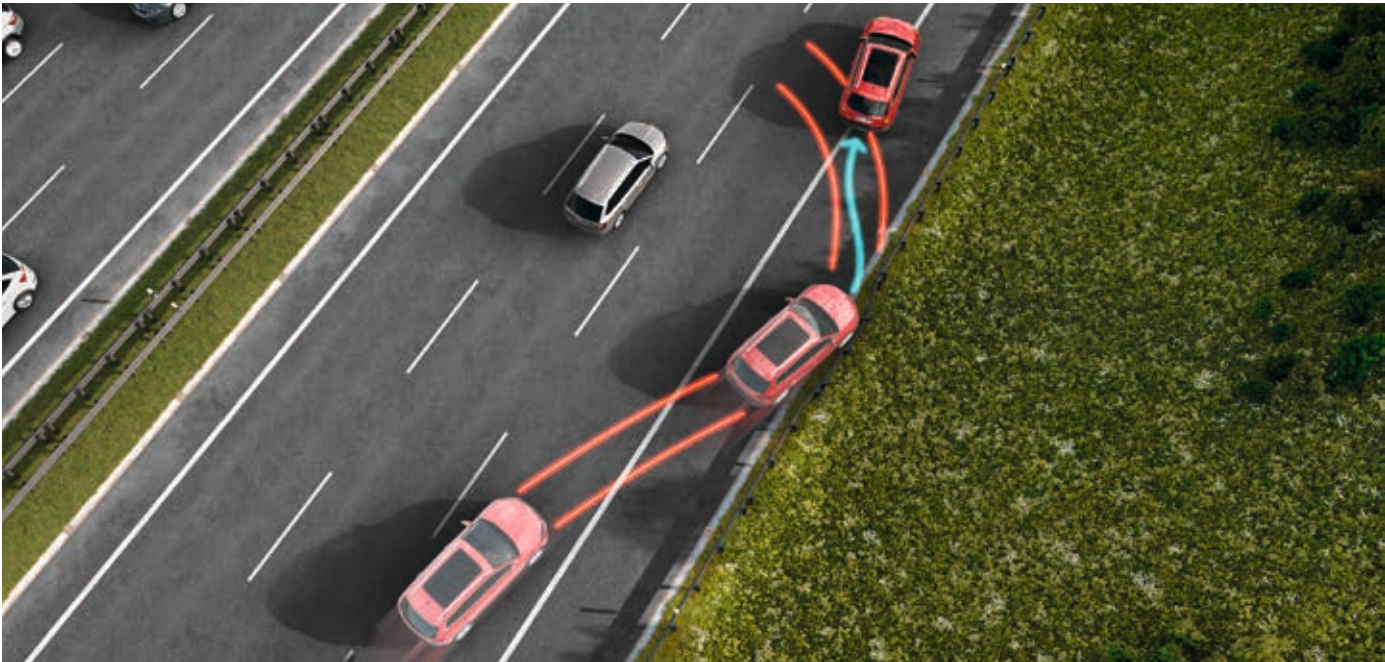
MULTI-COLLISION BRAKE In case of an accident, the Multi-Collision Brake starts braking to prevent further uncontrolled movement of the vehicle, thus reducing the likelihood of further collisions.
