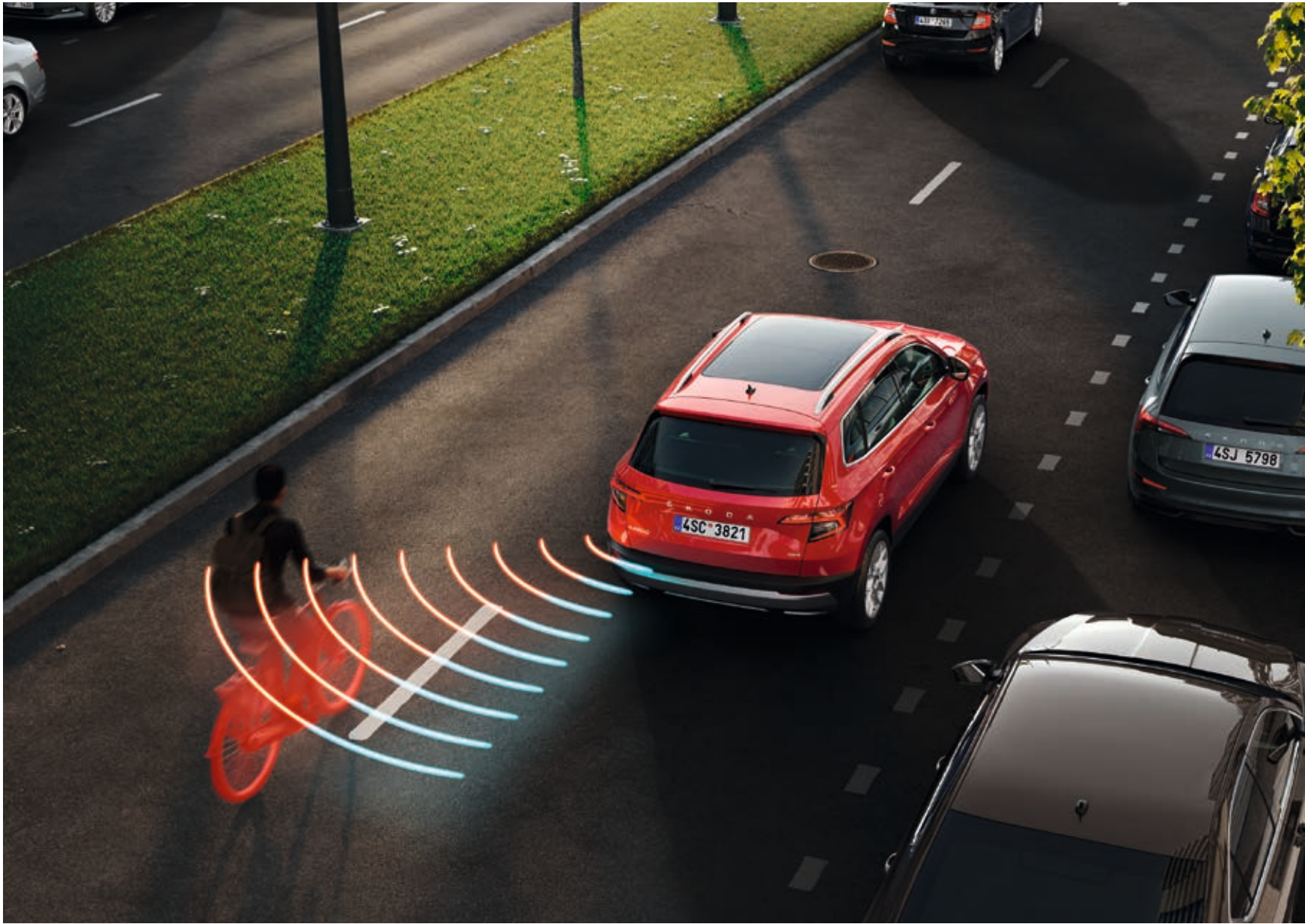
SIDE ASSIST Using radar sensors in the rear bumper, Side Assist (which can detect other vehicles and harder to see objects like cyclists up to 70 m away) monitors the areas behind and beside your car. Based on the distance and speed of the surrounding vehicles, it decides whether or not it should warn the driver.
